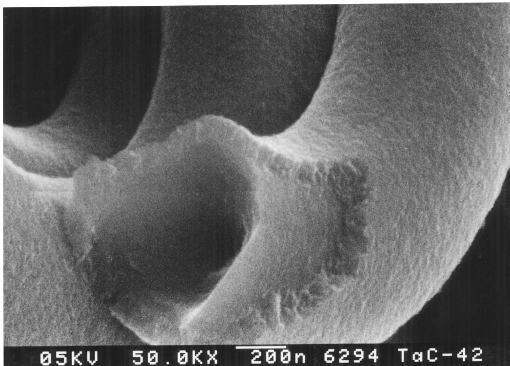
Figure 4 Ruptured cross section of the TaC micro-tubes. Reaction temperature: 1000°C, reaction time: 1 hr.
