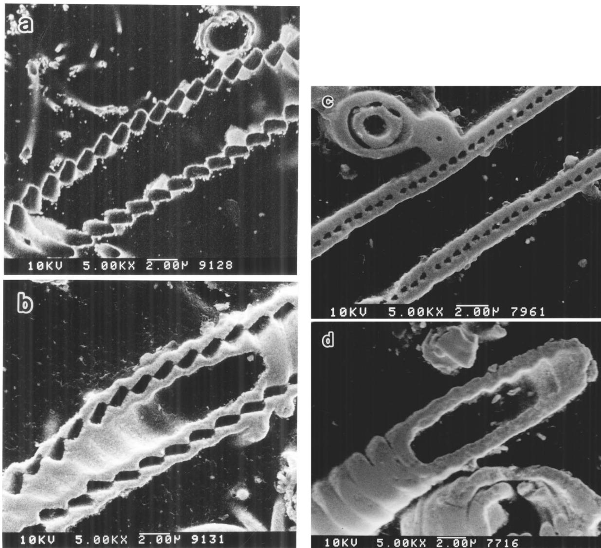
Figure 6 Polished cross section of the TaC micro-tubes. Reaction temperature: 1200°C, reaction time: (a) 0.5 hr, (b) 1 hr, (c) 2 hrs, (d) 3 hrs.
