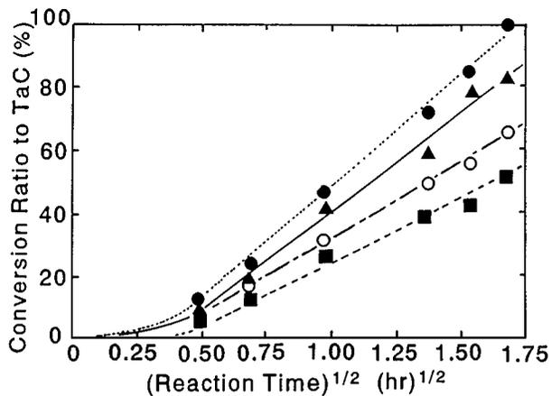
Figure 1 Relationship between conversion ratio of the carbon micro-tubes to TaC micro-tubes and square root of reaction time. Reaction temperature: (●) 900°C, (▲) 1000°C, (○) 1100°C, (■) 1200°C.
