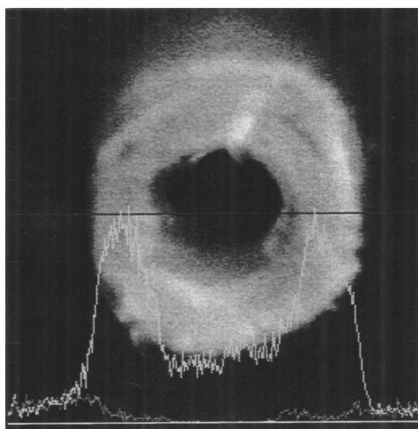
Figure 7 EPMA analysis on the polished vertical cross section of the TaC micro-tubes.
