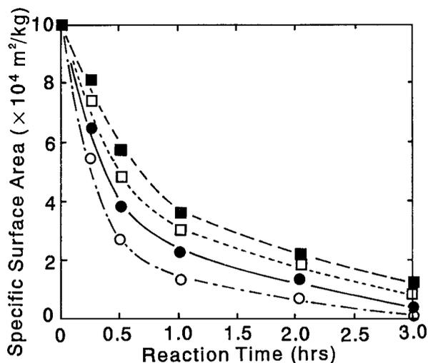
Figure 9 Relationship between specific surface area and reaction time. Reaction temperature: (■) 900°C, (□) 1000°C, (●) 1100°C, (○) 1200°C.
