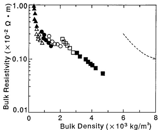
Figure 8 Relationship between bulk electrical resistivity and bulk density. (▲) source as-grown carbon coils. Conversion rate of the carbon micro-tubes to the TaC micro-tubes: (△) 23%, (●) 46%, (○) 69%, (□) 81%, (■) 100%. (-----) TaC powder.
