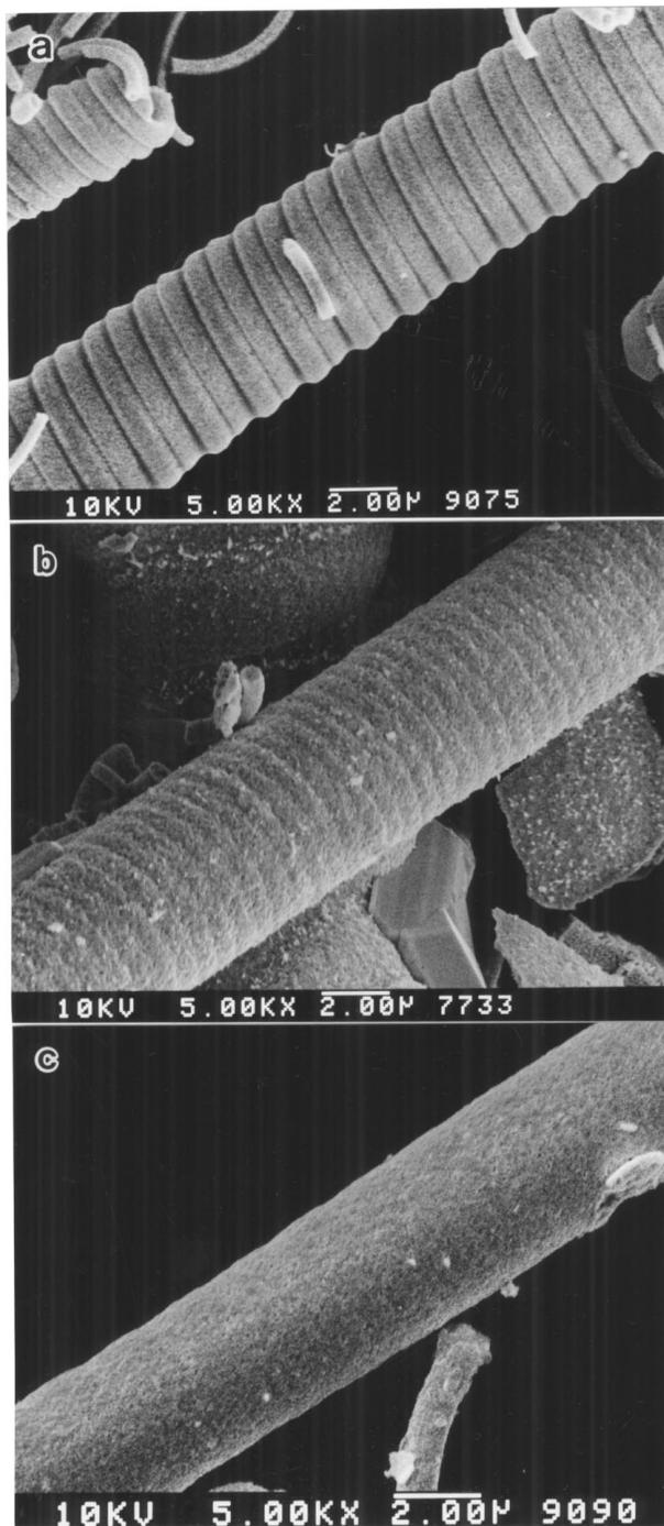
Figure 3 Surface morphology of the TaC micro-tubes. Reaction temperature: 1200°C, reaction time: (a) 1 hr, (b) 2 hr, (c) 3 hr.
