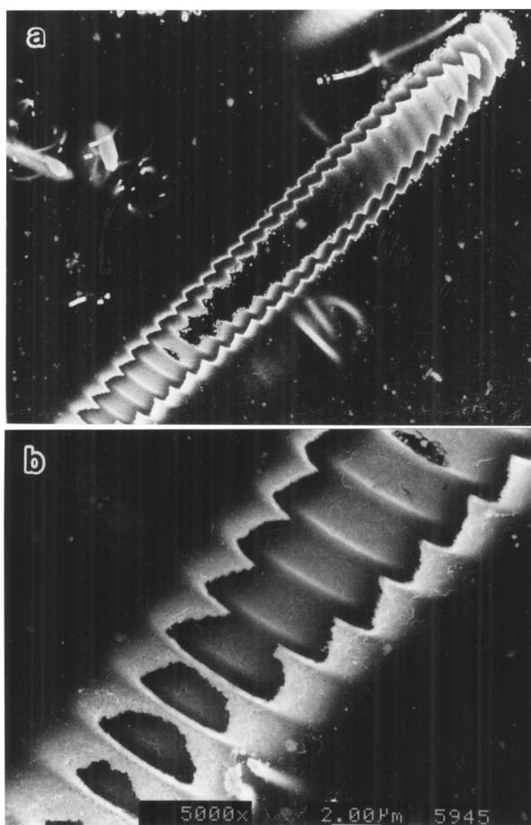
Figure 5 Polished cross section of the TaC micro-tubes (a) and the enlarged view (b). Reaction temperature: 1000°C, reaction time: 1 hr. The outer and inner white thin layer parts are the formed TaC layers, and the black and/or transparent part enclosed by the white part is the unreacted carbon micro-tubes.
