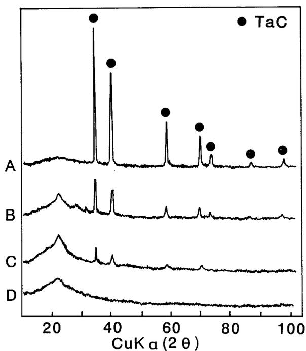
Figure 2 X-ray diffraction profiles. Reaction temperature: 1200°C, reaction time: (a) 3 hr, (b) 2 hr, (c) 1 hr, (d) source as-grown carbon micro-tubes.
